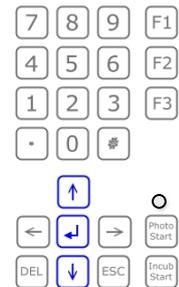
If you wish to work with a running number for the sample identification you have to enter a start number for the first sample to be measured. The MC 10<sup>plus</sup> suggests number one. (if an identification via Pat.-ID is required skip the next display).
