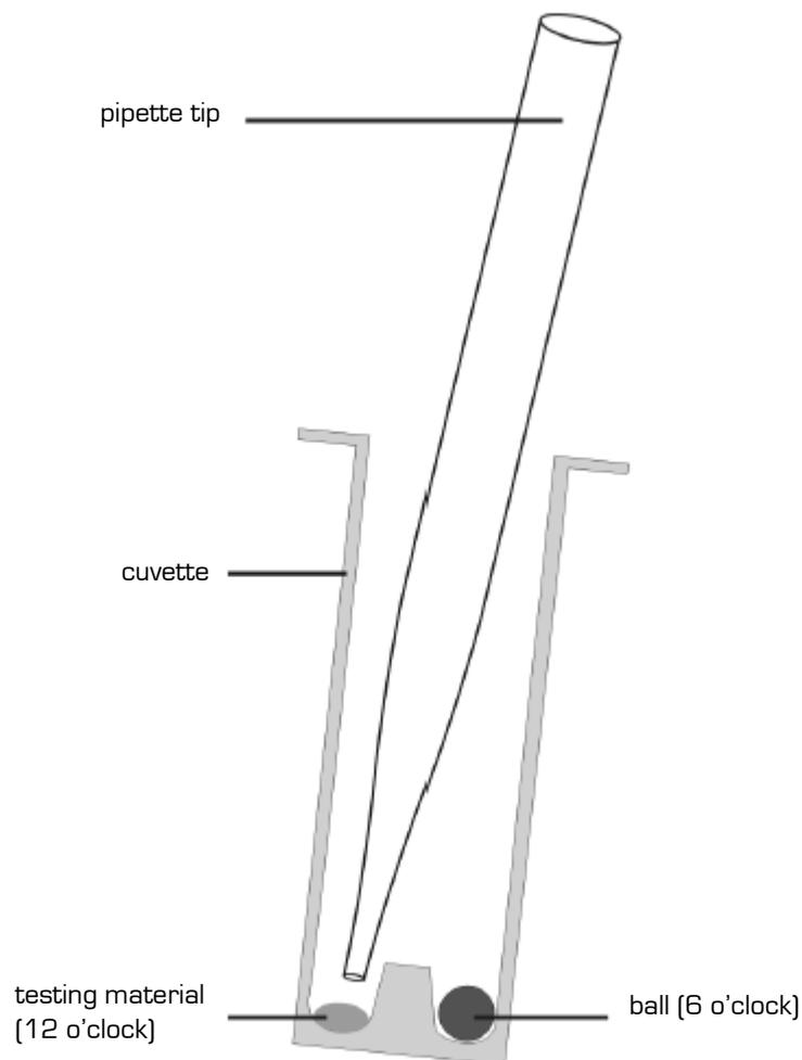
**4.4 Dispense of reagent 1 (microlitre pipette or Handystep pipette)**
