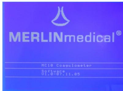
After approx. 15 sec. the display changes automatically from the welcome display to the start menu. The signal lamps do no longer light up.
