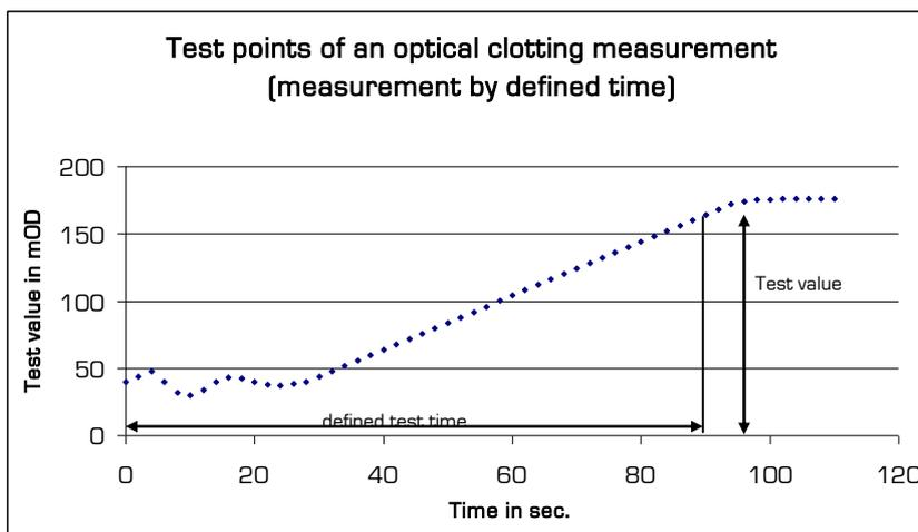
Ensure the correct kind of calculation resp. measurement when entering the test parameters. The correct test method is stated on the reagent package insert. For questions please approach your contact person, the reagent supplier or the company ABW.
