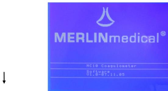
After approx. 15 sec. the display changes automatically from the welcome display to the start menu. The signal lamps do no longer light up.
