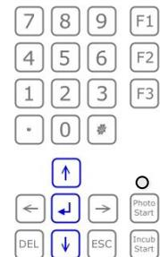
Here different parameter specifications can be determined. By selecting the parameter to be modified via the arrow keys and by confirming with ENTER you get into the display of the according parameter. Depending on the parameter following settings can be done:
